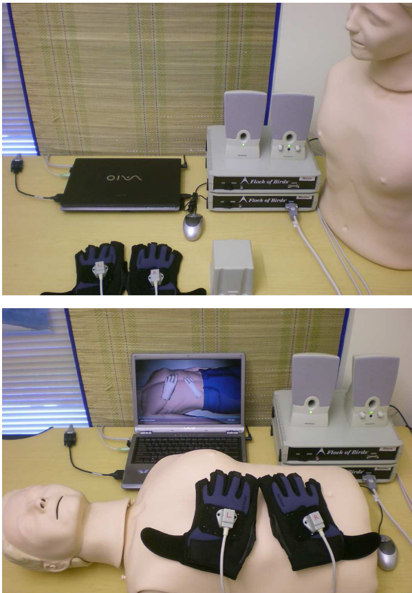
Figure 1. Anne Torso , a realistic lifesize CPR trainer, from Laerdal [1], augmented with a tangible user interface. System components: the manikin object, Flock of Birds tracking system with two sensors Velcroed onto sports gloves, laptop PC, speakers. Below: the manikin in working position for physical examination, with a debug view of the 3D models on the laptop screen.
